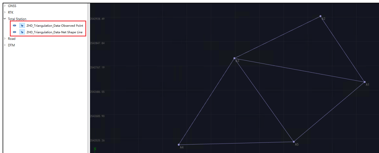
Figure 13-1-7 Total Station Layer Management
